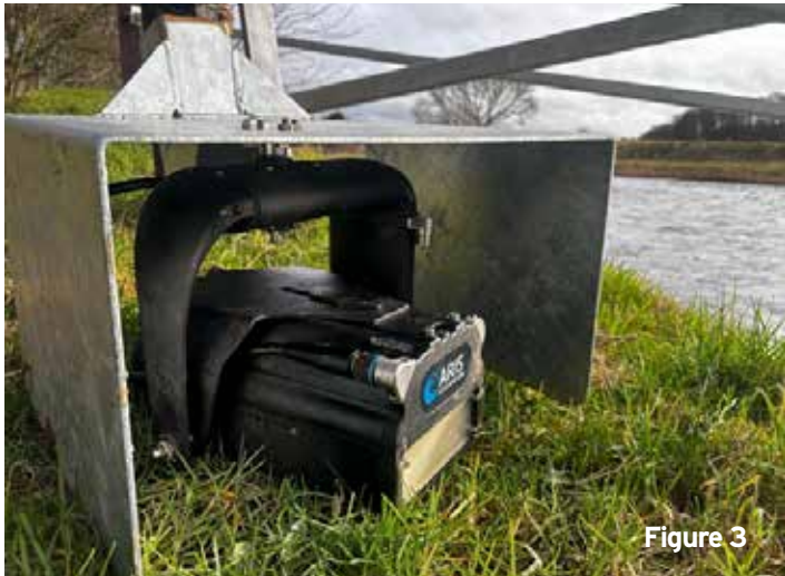
Fig 1. View upstream with the ARIS deployed from the right bank on adjustable protection arm.
