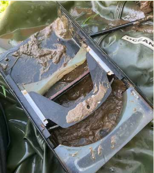
The quantity of sediment being washed down the river is well illustrated by the build of silt inside the ARIS SONAR fish counter at Montcoffer. This occurred over just a couple of days following heavy thunderstorms and severe run off.
